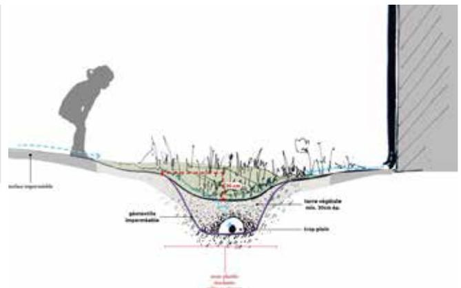
Wet swale with infiltration layer, connected to the drainage .
